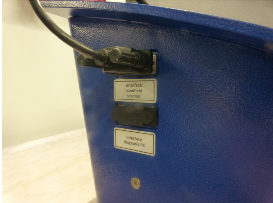
Connection of fixed scanner SVP-5
