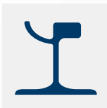
Grooved rail (tram)
