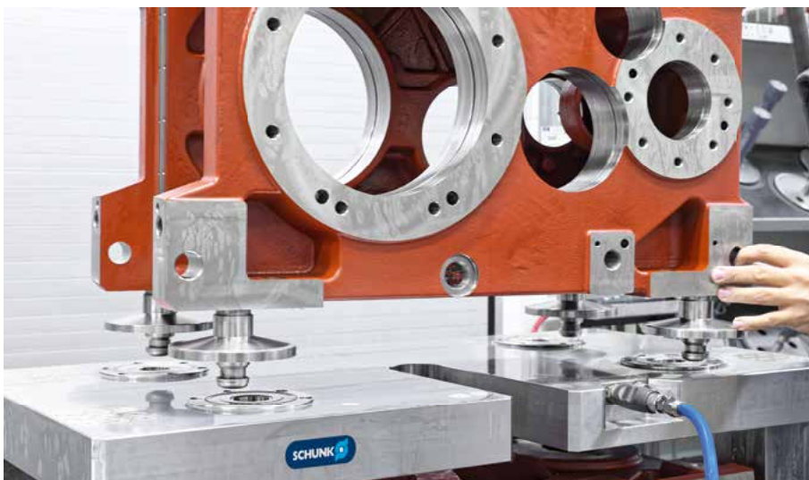
The lower level of the fixture is clamped with low deformation using magnetic clamping technology. The upper clamping point is designed with VERO-S quick-change pallet technology. This makes the workpiece change quick, ergonomic, and precise. (Detail: VERO-S pin in the quick-change pallet module)
