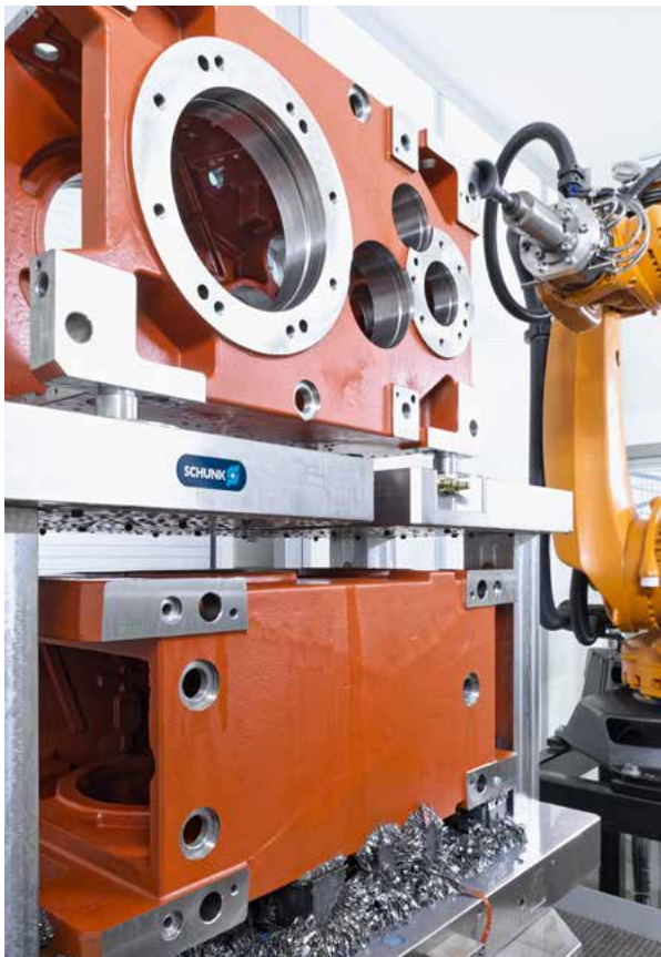
Synergy of clamping technologies: On the lower level, low-deformation clamping using magnets. On the upper level, direct clamping in the quick-change pallet system.
