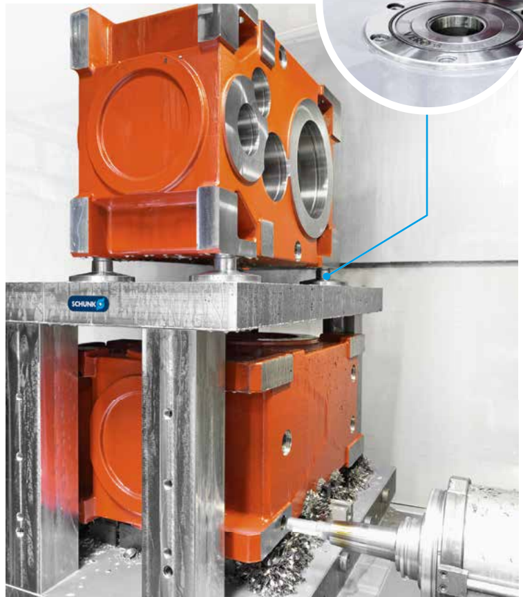
The lower level of the fixture is clamped with low deformation using magnetic clamping technology. The upper clamping point is designed with VERO-S quick-change pallet technology. This makes the workpiece change quick, ergonomic, and precise. (Detail: VERO-S pin in the quick-change pallet module)
