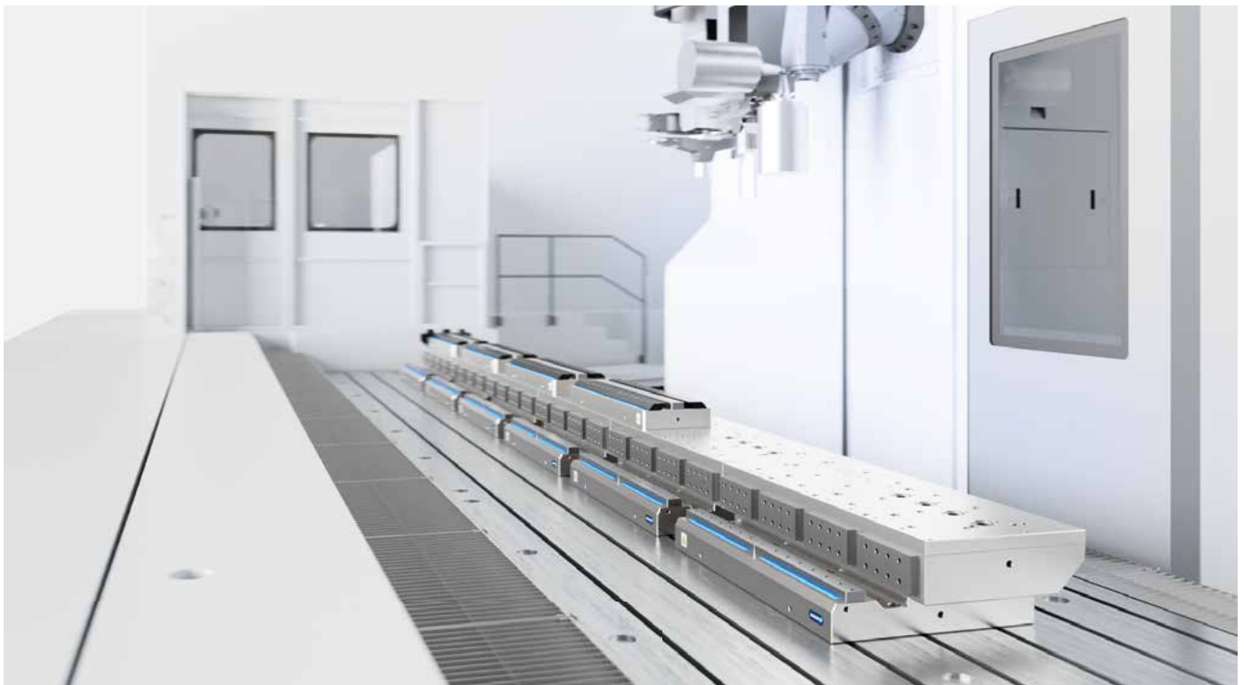
Machining of the groove in a solid rail, cutting depths of up to 47 mm in one cut, the vertical clamping ensures optimal chip removal, this increases the machining quality while reducing tool wear at the same time.
