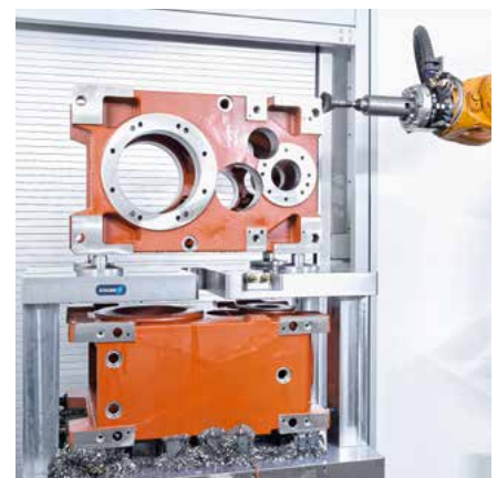
Left: Exchanging workpieces on the upper clamping level only takes a few seconds with the SCHUNK VERO-S quick-change pallet system. Right: Robot-assisted deburring of components
