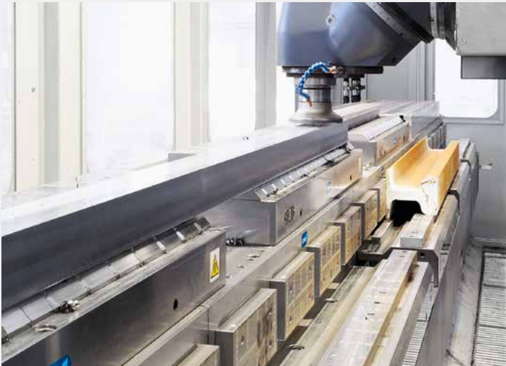
Before groove milling, the track elements are processed with the face-milling cutter. The workpieces are clamped on the foot and on the side of the rail head.
