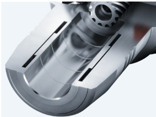
Dirt grooves for reliable torque transmission
