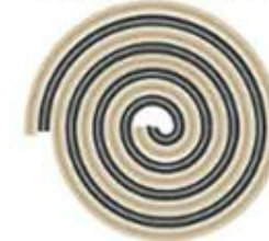
c) Cylindrical winding
