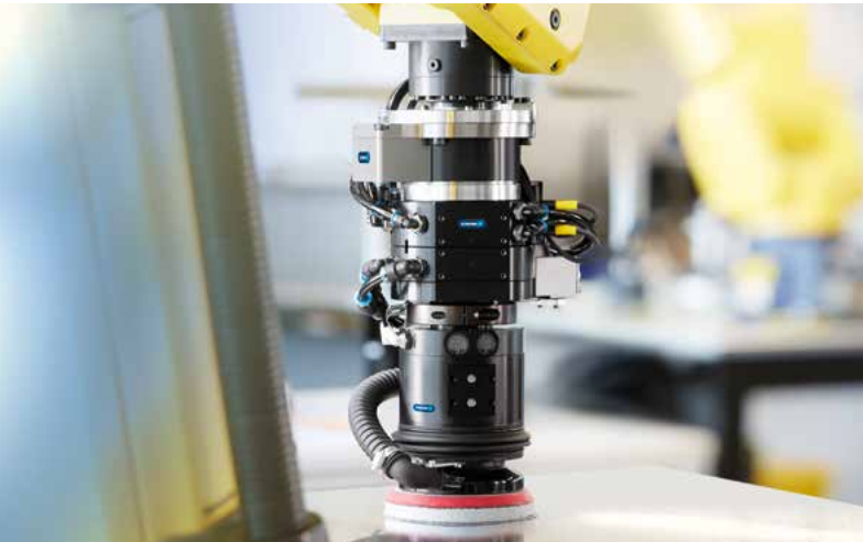
Automated grinding with the robot
