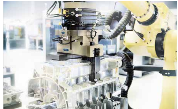
Handling of motor blocks
