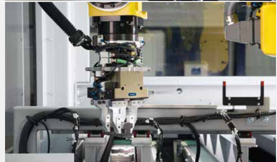
Change systems & feed-through modules
