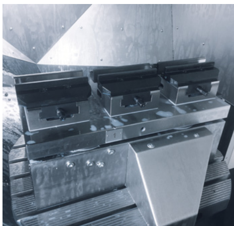
5-Achs Backe Breite 125 fest H=33 5-axis jaw width 125 fixed H=33
