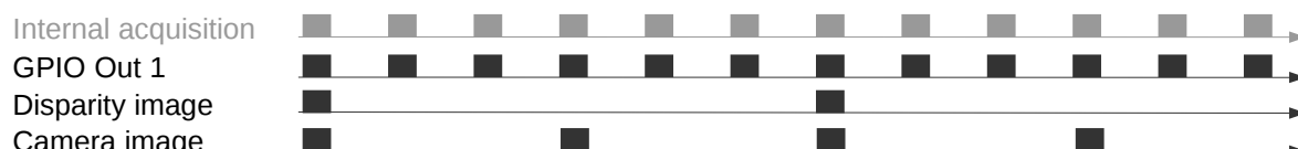
Fig. 6.27: Example of using the ExposureActive mode for GPIO Out 1 with a user-defined frame rate of 8 Hz. The internal image acquisition is always 25 Hz. GPIO Out 1 is HIGH for the exposure time of every image. A disparity image is computed for camera images that are sent out via GigE Vision according to the user-defined frame rate.
