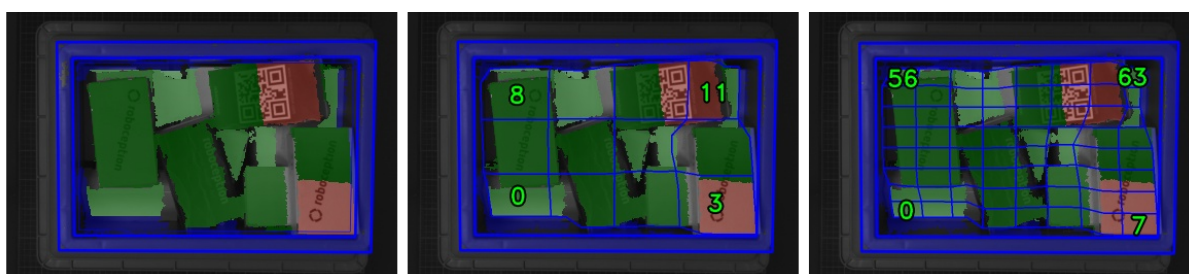
Fig. 7.11: Visualizations of the load carrier filling level: overall filling level without grid (left), 4x3 grid (center), 8x8 grid (right). The load carrier content is shown in a green gradient from white (on the load carrier floor) to dark green. The overfilled regions are visualized in red. Numbers indicate cell IDs.
