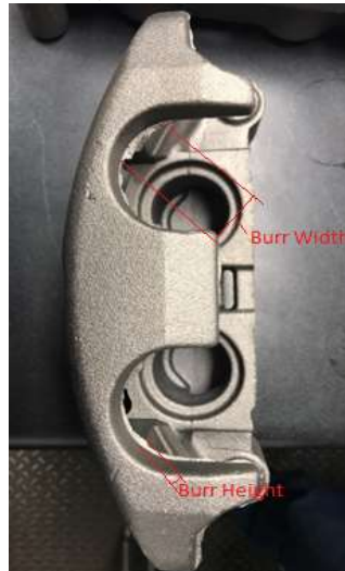
Burr Height and Burr Width Defined
