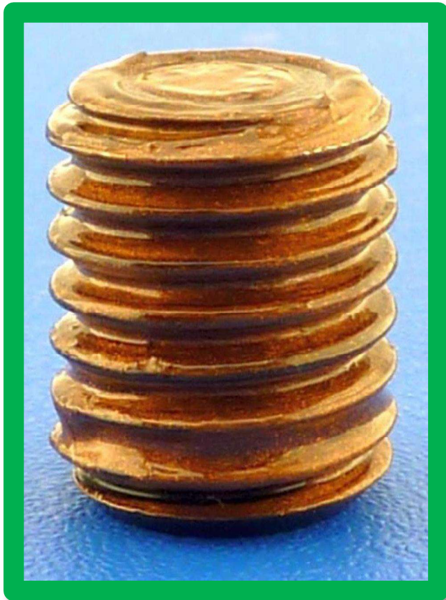
Optimal lubrication condition (Condition after clamping)
