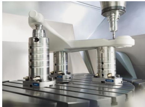
Direct workpiece clamping
