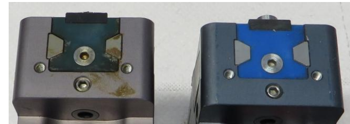
Discoloration by temperature impact
