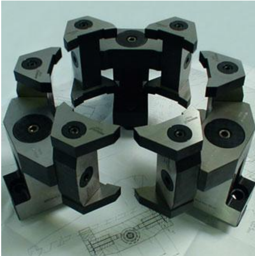
12 clamping points on two clamping levels designed to permit an axial and radial alignment of the clamping system of the component
