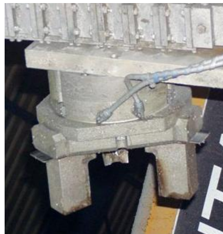
Figure 2: Gripper with dust cover under operating conditions
