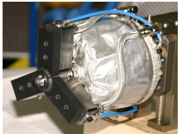
Figure 2: Textile heat protection cover for a centric gripper
