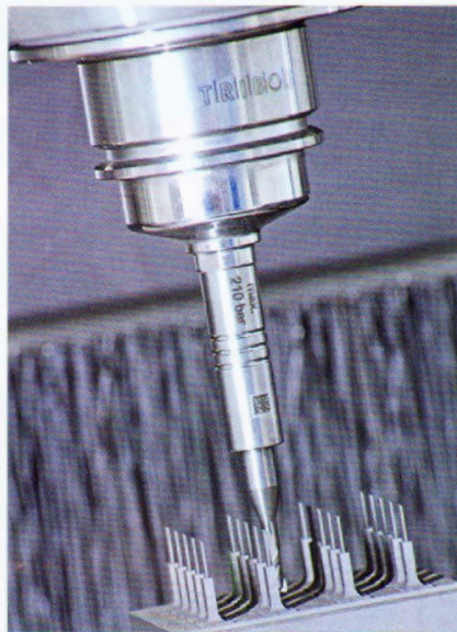
4 | By using TRIBOS-S, extremely fine contours can be process-reliably machined when graphite machining
