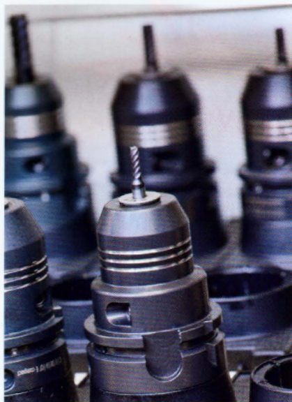
3 | The price-attractive hydraulic expansion toolholder TENDO E compact can be used for applications from volume machining up to finish machining
