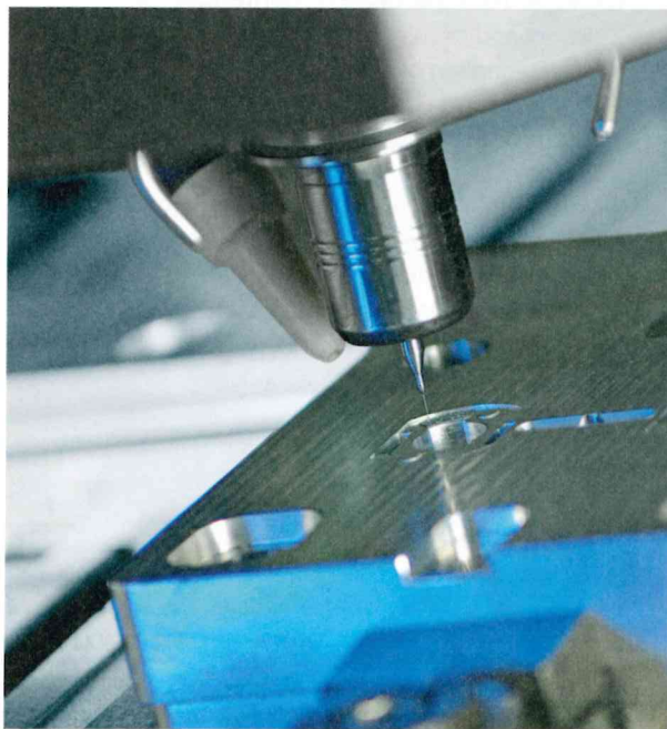
2/ In the mold making industry the Tribos-RM is used for presenting fine structures very precisely
