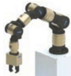
7 DOF LWA-Arm with 3 kg payload*
