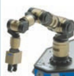
7 DOF LWA-Arm with 10 kg payload*
