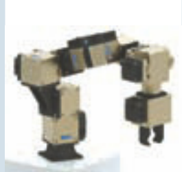
6 DOF PBA-Arm with 3 kg payload*
