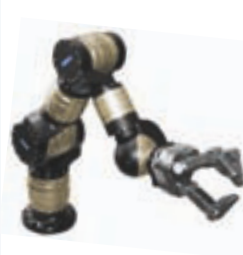
7 DOF LWA4-Arm with 10 kg payload*
