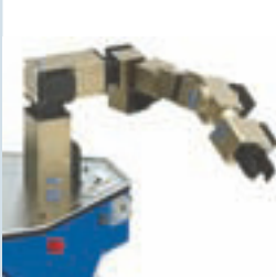
7 DOF LWA-Arm with 10 kg payload*
